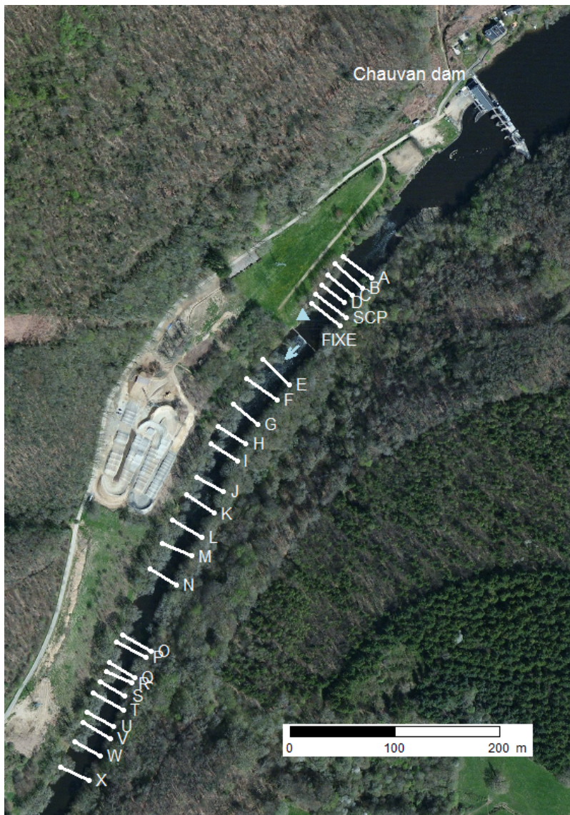
Figure 2.5: Location of each cross-section (OpenStreetMap). The blue triangle shows the EDF-DTG hydrometric station.
